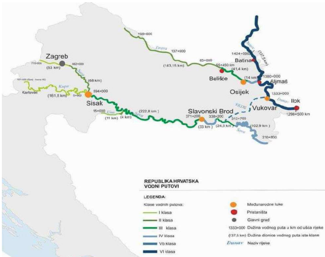
Figure 3.8 The network of inland waterways of the Republic of Croatia (Source: The Ministry of the Sea, Transport and Infrastructure)
